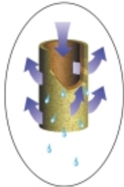
Figure 1 Dual Layer Filter Element - long life and high efficiency
