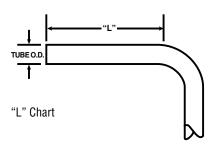
Note: You will need a **minimum straight length** of tubing ahead of any bend to fit into the pre-setting tool. See the "L" dimension in the chart for each tube O.D. size.
