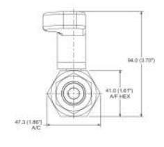
**Standard product specification**: PTFE packing with PTFE seats, 10mm ball bore 6,000 psig (414 barg). **Standard product specification**: PTFE packing with PEEK seats, 10mm ball bore 10,000 psig (689 barg).
