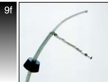
9f Remove excess nichrome wire and separate bus wires.
