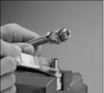
Using Parker Hoze-Oil or an SAE 20 lubricating oil, lubricate nipple and socket threads. For stainless steel fittings use Parker 702 Oil or a molybdenum type lubricant. For hose used in oxygen service lubricate using a non-oil based soap solution.
