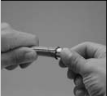
Verify tube butts against inside shoulder of sleeve.
