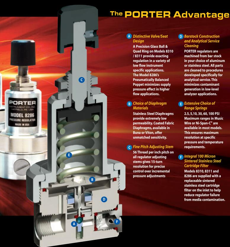
Design A Precision Glass Ball & **Quad Ring on Models 8310** / 8311 provide exacting regulation in a variety of low flow instrument specific applications. The Model 8286's **Pneumatically Balanced** Poppet minimizes supply pressure effect in higher flow applications.
