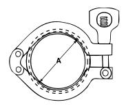
13MHHM - Heavy Duty Clamp Double Pin Hinge
