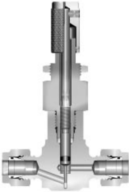
Figure 1: NM/NL Series Metering Valve with Knurled Handle Cross Sectional View
