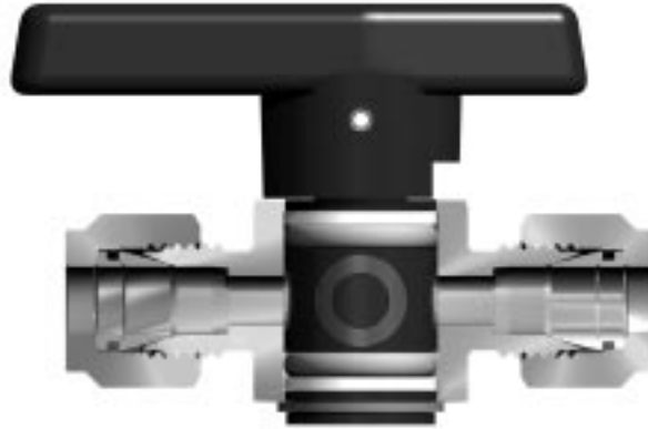
Figure 1: PR Series Rotary Plug Valve Cross Sectional View
