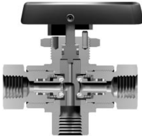
Figure 1: HB Series Ball Valve Cross Sectional View
