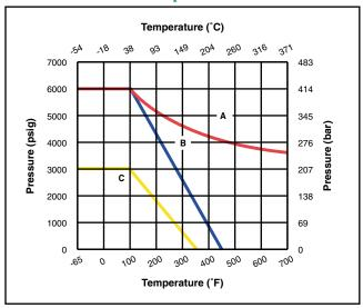
**Legend:** A - Grafoil® packing with R stem; B - PTFE packing with R stem; C - PTFE packing with K stem.
