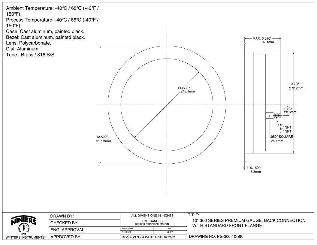
Ambient Temperature: -40°C / 65°C (-40°F / 150°F). Process Temperature: -40°C / 65°C (-40°F / 150°F). Case: Cast aluminum, painted black. Bezel: Aluminum. Lens: Polycarbonate. Dial: Aluminum. Tube: Brass / 316 S/S. Movement: Brass / 304 S/S. Socket: Brass / 316 S/S. Accuracy: +/- 0.5% of full scale. Enclosure: IP52.
