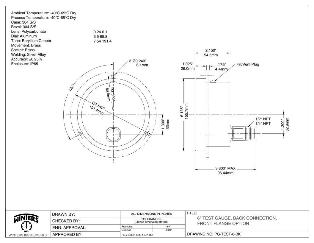
Ambient Temperature:  $-40^{\circ}$ C-65°C Dry Process Temperature:  $-40^{\circ}$ C-65°C Dry Case: 304 S/S Bezel: 304 S/S Lens: Polycarbonate Dial: Aluminum Tube: Beryllium Copper Movement: Brass Socket: Brass Welding: Silver Alloy Accuracy:  $\pm 0.25\%$ Enclosure: IP65
