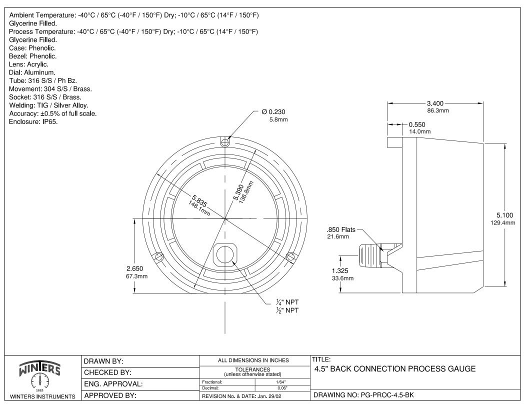
Ambient Temperature: -40°C / 65°C (-40°F / 150°F) Dry; -10°C / 65°C (14°F / 150°F) Glycerine Filled. Process Temperature: -40°C / 65°C (-40°F / 150°F) Dry; -10°C / 65°C (14°F / 150°F) Glycerine Filled. Case: Phenolic. Bezel: Phenolic. Lens: Acrylic. Dial: Aluminum. Tube: 316 S/S / Ph Bz. Movement: 304 S/S / Brass. Socket: 316 S/S / Brass. Welding: TIG / Silver Alloy. Accuracy: ±0.5% of full scale. Enclosure: IP65.
