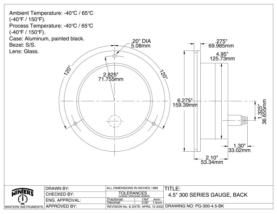
Ambient Temperature: -40°C / 65°C (-40°F / 150°F). Process Temperature: -40°C / 65°C (-40°F / 150°F). Case: Steel, painted black. Bezel: Aluminum. Lens: Glass. Dial: Aluminum. Tube: Brass / 316 S/S. Movement: Brass / 304 S/S. Socket: Brass / 316 S/S. Accuracy: +/- 0.5% of full scale. Enclosure: IP52.
