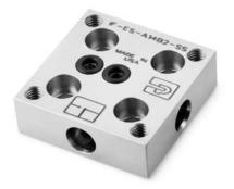
All Parker IntraFlow™ fittings are permanently marked with the part number, flow schematic and material heat traceability code for easy identification during assembly and when servicing in the field. 1/8" diameter internal flow paths are precision machined at the intersections to minimize dead volume. Slip fit counterbores with a lead-in chamfer retain intra-connecting pressure connectors.
